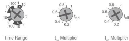
In the above figure:  $t_{on} = 10h \times 0.5 = 5 \text{ hour}$      $t_{off} = 10h \times 0.1 = 1 \text{ hour}$
