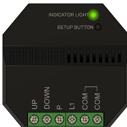
Green flashing Indicator Light Touchlink Commissioning Mode
