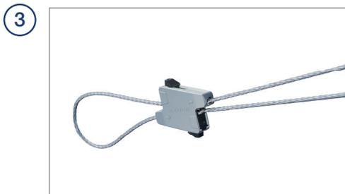
3 The loop is now secure. Ensure at least 100mm of tail wire exits the hanger and the inclusive angle is <math><60^\circ</math>.
